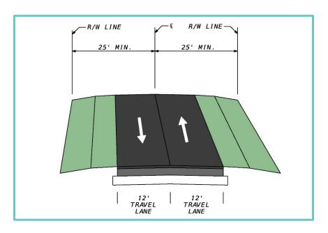
Figure 2-2 | Typical Section – Existing Lena Road from 41st Avenue East to SR 64
