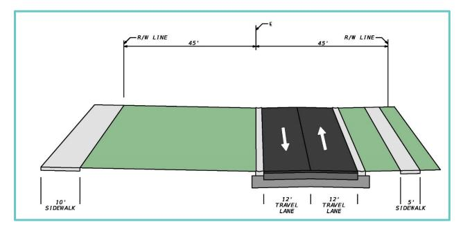
Figure 2-1 | Typical Section – Existing Lena Road north of SR 70 to cul-de-sac
