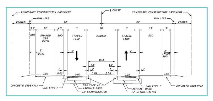
Figure 4-3 | Build Typical Section 2
