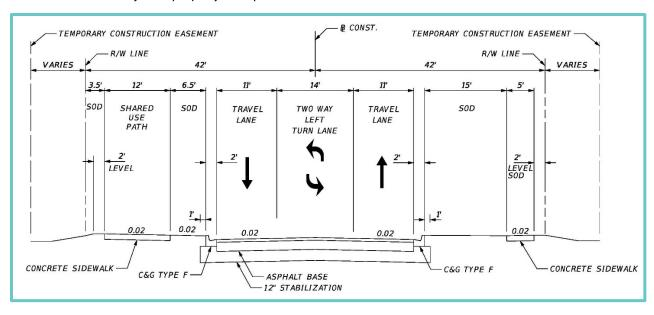
Figure 4-4 | Build Typical Section 3
